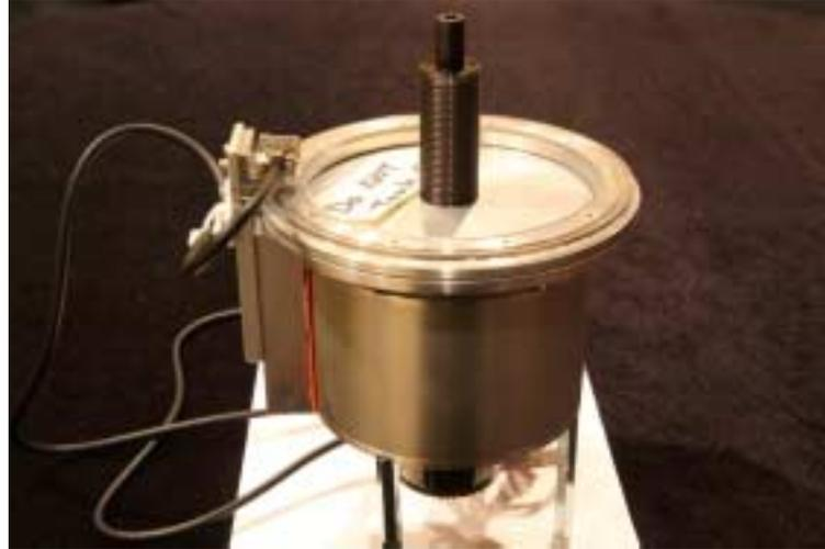
**Figure 4: Motor testbed to measure 12-bit magnetic encoder accuracy**
