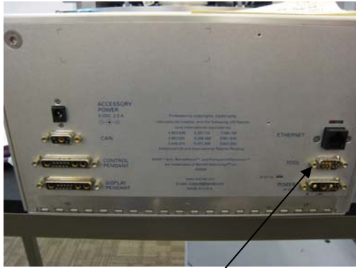
Male 9-pin D-Sub connector labeled “TOOL”
