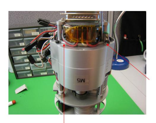
Remove the two screws that hold the puck to the wrist using a 2mm hex driver, as shown, One screw will have a lock washer on it, while the other has the ground line from the puck. Make sure you put these back in the same fashion.
