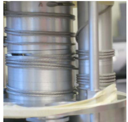
Figure 11 – Taping the M5 Stage-3 Lower-Pinion
