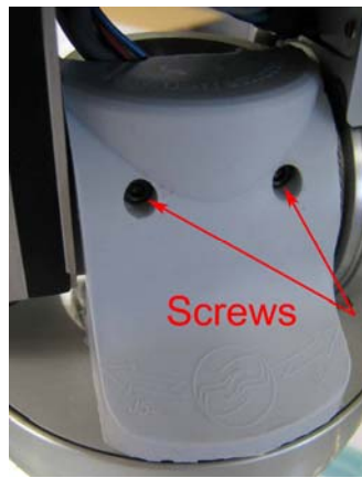
Figure 6 -- RTV rubber shroud.
