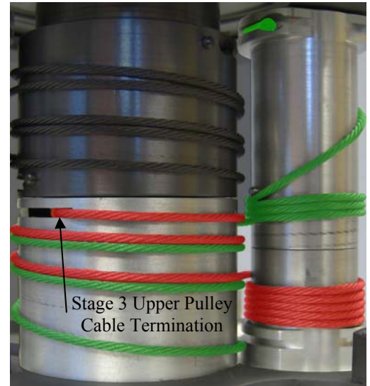
Figure 10 – M5 Stage-3 Cables (color-enhanced)
