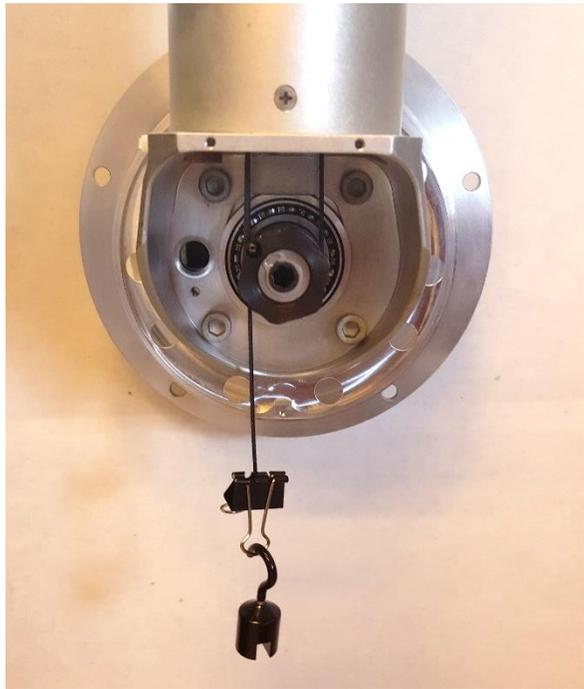
5. Wrap Cable B6235 around Pulley A 5 times and position the mini clap as shown. The cable and weight should no longer be visible at the one-way tensioning clutch.
