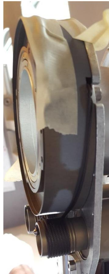
12. Take Cable B6235 and secure to bottom anchor slot of Pulley B with tape and wrap around 1 ½ times.
