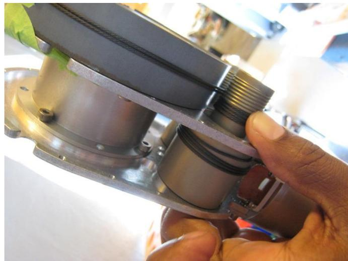
10. Take Cable B4504 and match the two termination ends together. Attach the middle portion of Cable B4504 to the bottom anchor on stage 2 Pulley C.
