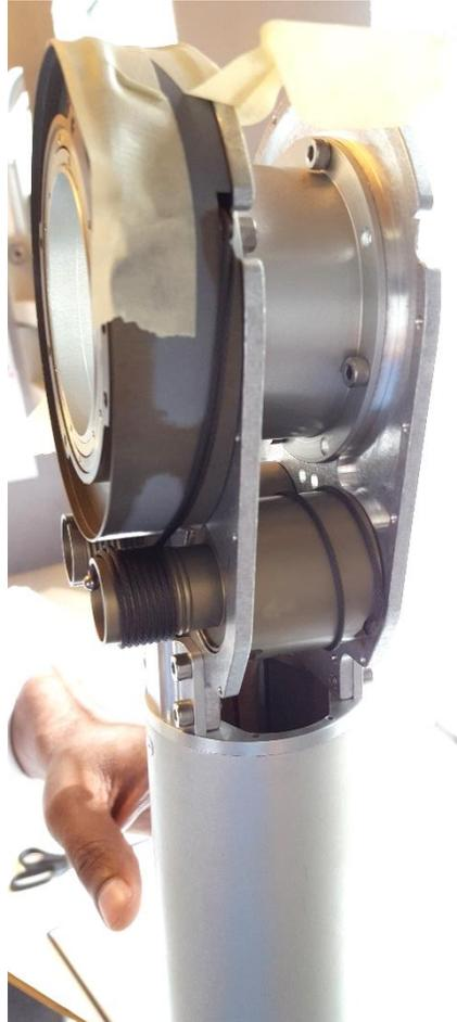
13. Put the remaining Cable B4504 down the shaft of the Inner Link. The remainder of the cable should show by the one-way tensioning clutch (Both Cables B6235 should be seen).
