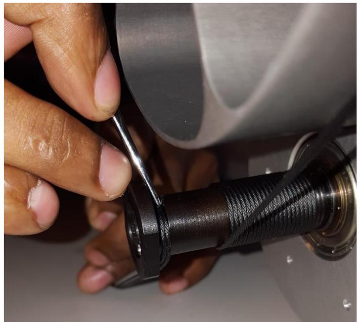
8. Insert the 4mm hex key into the one-way tension clutch and hold the key while holding tension on the cable. Rotate the end of Pinion 1 by hand until the cable has no slack.
