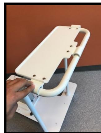
7. Fasten the lifting column to the T-plate using 4 socket head screws and cover them with the 4 white screw caps.
