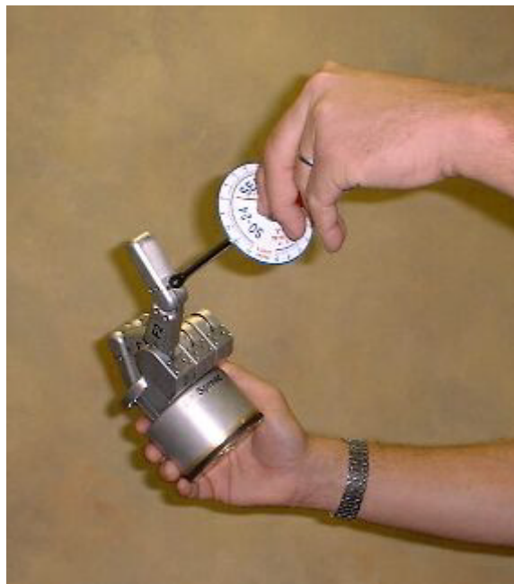
Figure 9 - Pretensioning the Tendon Cable
