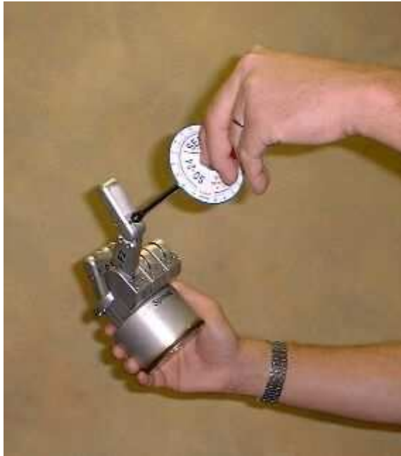
Figure 9 - Pretensioning the Tendon Cable
