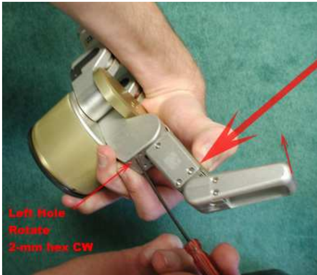
Figure 19 - Manual Torque Switch Activation
