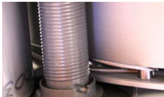
Figure 26 – Wrap behind Motor Pinions
