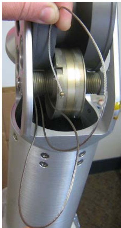
Figure 60 – Inserting the Terminations into the Side-A Anchors
