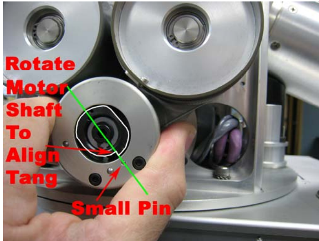
Figure 10 -- Align motor with tang to remove cylinder cup.
