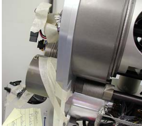
Figure 47 – Securing the Stage-1-Pulley
