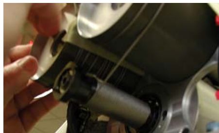
Figure 51 – Wind 1+1/2 Times onto Pulley
