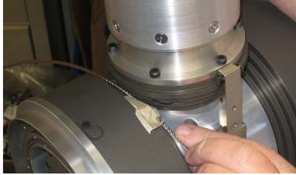
Figure 73 – Sliding the Level-1-Cable down the Side-A Gap
