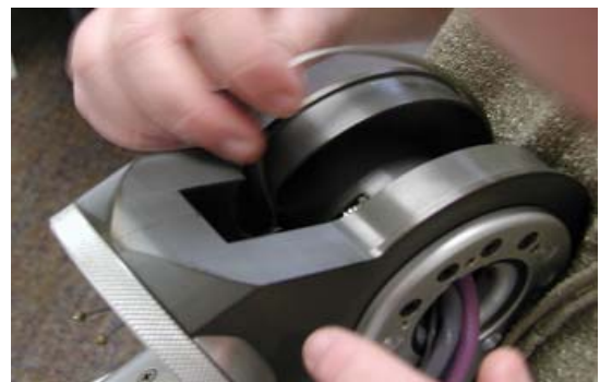
Figure 64 – Looping Cable around Side-B Anchor
