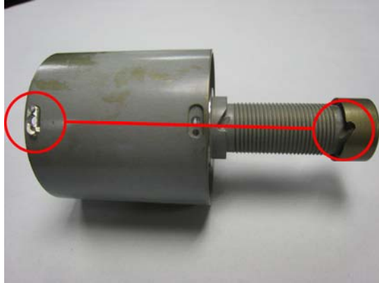
Figure 28 – First use the Pinion Anchor that is in line with the Pulley Anchor.
