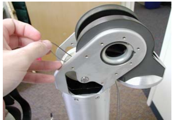
Figure 63 – Feeding the U-loop between Pinion and Pulley
