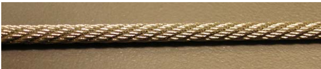
Figure 1 -- Healthy drive cable before installation
