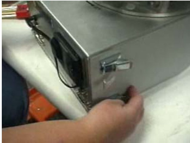
Figure 15 -- Removing four clasps that secure the U-shaped plastic base cover.
