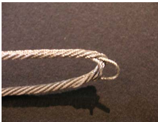
Figure 2 -- Typical appearance of a cable damaged during handling
