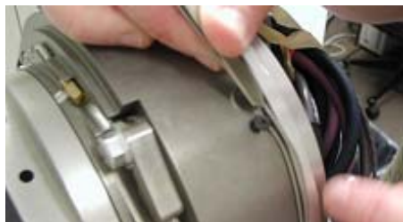
Figure 46 – Installing Cable in Outboard Loop-Anchor-Groove
