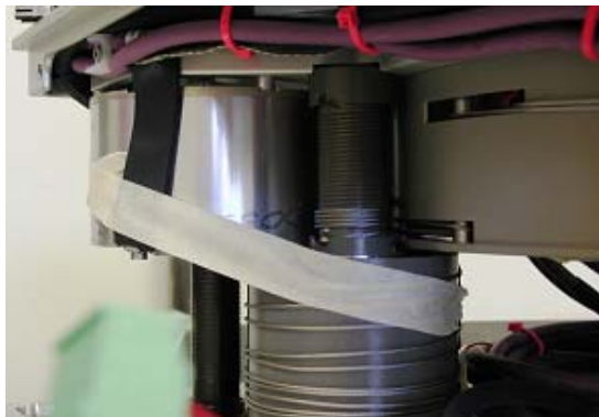
Figure 34 – Securing the Side-A Stage-1-Pulley
