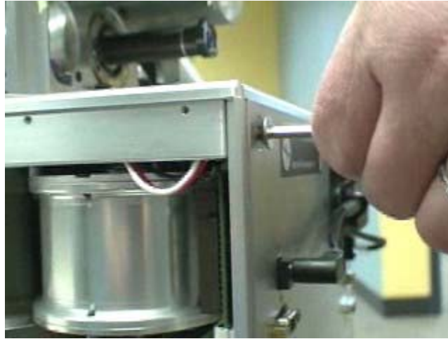
Figure 17 -- Remove single screw from backplate with 4-mm hex wrench.
