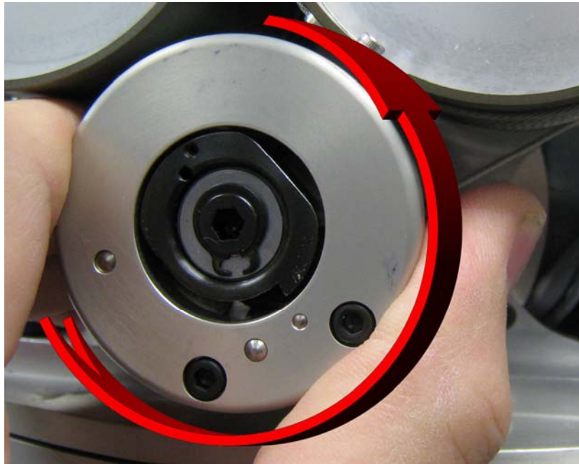
Figure 12 -- Removing old-type tensioner.
