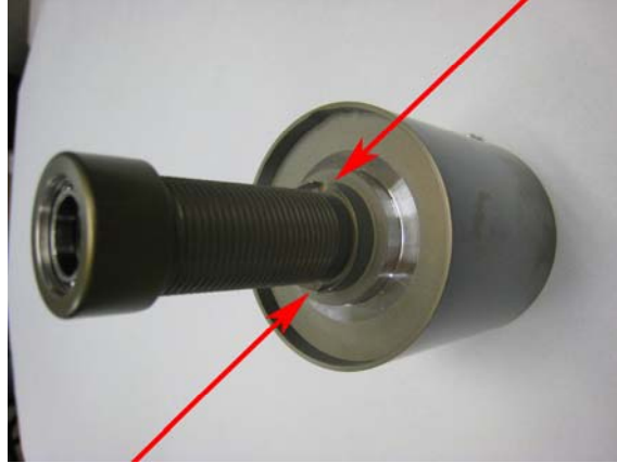
Figure 32 -- Twin termination anchors at Outboard end of pinion.
