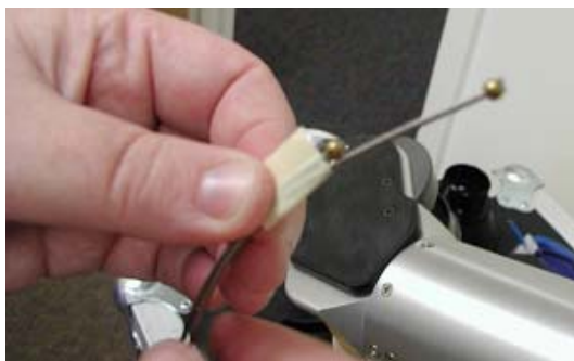
Figure 45 – Uneven Stage-2-Cable Ends
