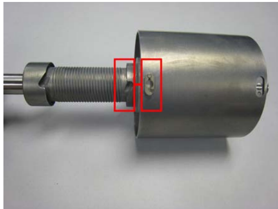
Figure 33 -- First use pinion anchor that is aligned with the Pulley anchor.
