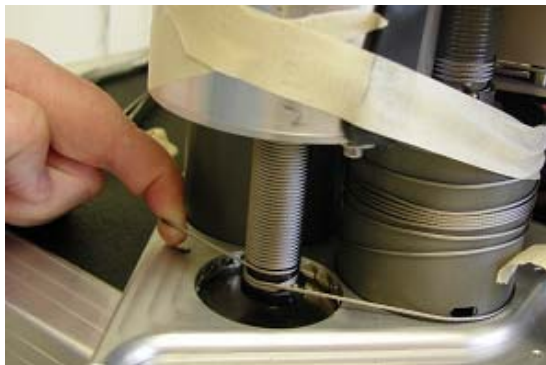
Figure 36 – Using Finger to Maintain Tension
