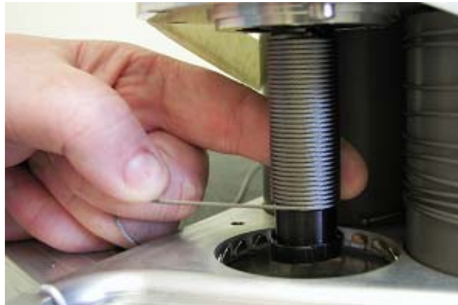
Figure 35 – Wrapping Stage-1-Cable onto Pinion
