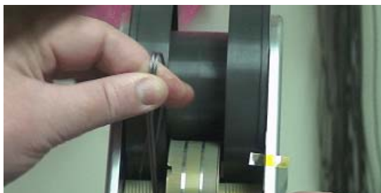
Figure 60 – Inserting the Terminations into the Side-A Anchors
