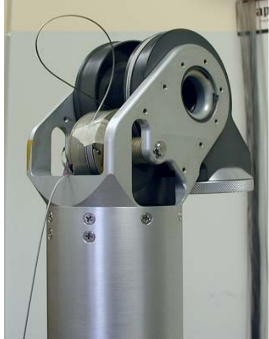
Figure 68 – Wrapping Side-B Cable 6 Times
