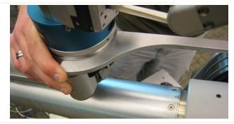
Rotate Joint 7 of the WAM counter clockwise until it is up against its joint stop. Insert the spanner pin into one of the two holes on the WAM's screw ring. Hold the wrist with a finger on the spanner to prevent the pin from popping out.
