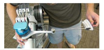
Use the same method to tighten the hand to the FT Sensor, torqueing down both sides of the FT screw ring.
