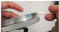
Unscrew the cap off of the Tool Oil syringe, lightly saturate a cotton swab tip with the Tool Oil and run it over the male threads of the Force Torque Sensor as shown. Soak up any excess oil by running a dry cotton swab over the threads. The oil layer should be a very thin sheen, and should not drip.
