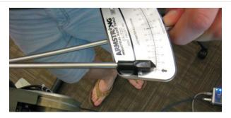
Holding the beam torque wrench by the ball handle, carefully tighten the screw ring to the level indicated by the black arrow on the dial. (Approximately 12 N-m of torque about the threads)
