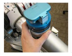
Repeat the same steps with the BarrettHand. Oil the male threads on the base of the BarrettHand. Clean the outer edge of its bottom surface and the outer edge of the Force Torque Sensors top plate with alcohol.
