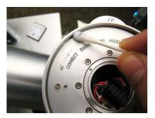
Lightly saturate a cotton swab tip with the alcohol and use it to wipe clean the outside edge of the bottom surface of the Force Torque Sensor as well as the outside edge of the WAM's tool plate. Make sure to remove any oil residue off of these surfaces. Use multiple swabs if necessary.
