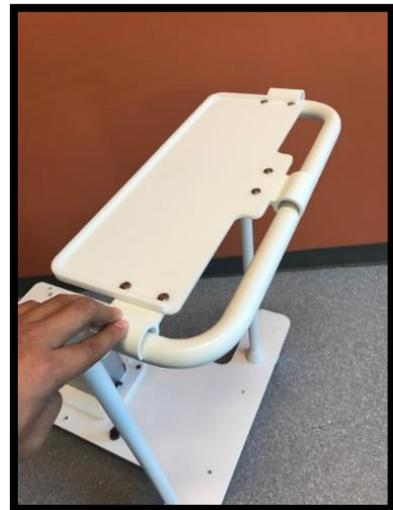
6. Fasten the lifting column to the T-plate using 4 socket head screws and cover them with the 4 white screw caps.
