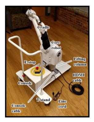
3. Fasten the handle onto the T-plate using the button (dome) head screws and verify its security.
