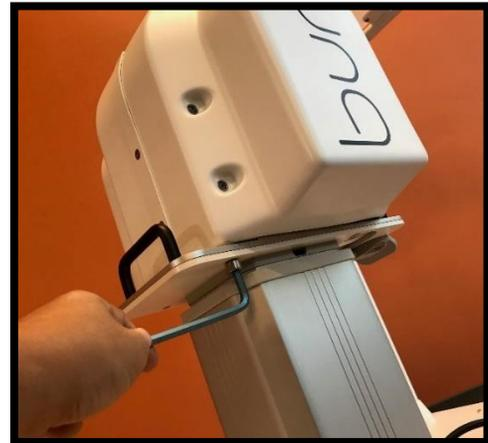
8. Place the console rubber legs on the 4 small screw heads with the BURT logo facing away from the lifting column.
